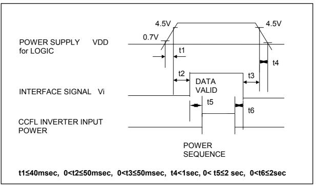
\* Set 0 Volt Vi(t)  $\leq$  V<sub>DD</sub>(t) Here Vi(t), V<sub>DD</sub>(t) indicate the transitive state of Vi, V<sub>DD</sub> when power supply is turned ON or OFF
