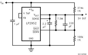
\* Turns ON at  $V_{IN} = 5.87V$ Turns OFF at  $V_{IN} = 5.64V$ (for component values shown)
