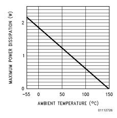
FIGURE 3. Power Derating Curve for LP2953AMJ
