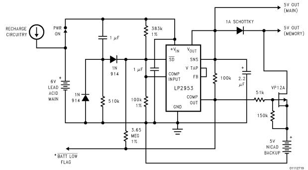
The circuit switches to the NI-CAD backup battery when the main battery voltage drops below about 5.6V, and returns to the main battery when its voltage is recharged to about 6V.
