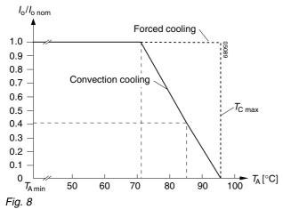
Output current derating versus temperature for -7 and -9 units.
