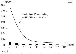
Harmonic currents at the input, IEC/EN 61000-3-2, class D.  $U_i = U_i \text{ nom}$ ,  $I_0 = I_0 \text{ nom}$ .
