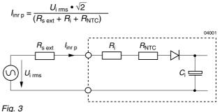
Equivalent circuit diagram for input impedance.
