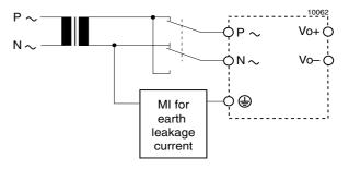
Fig. 29 Test set-up
