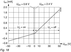
Typical inhibit current I<sub>inh</sub> versus inhibit voltage U<sub>inh</sub>
