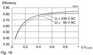
Efficiency versus load at Ui; 230 V AC and 85 V AC
