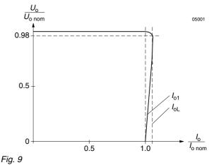
U<sub>o1</sub> vs. I<sub>o1</sub> (typ.) of single output units
