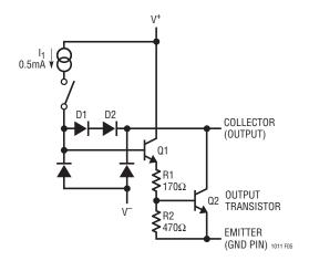
Figure 5. Output Transistor Circuitry
