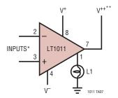
\*INPUT POLARITY IS REVERSED WHEN USING PIN 1 AS OUTPUT \*\*V\*\* MAY BE ANY VOLTAGE ABOVE V<sup>-</sup>. PIN 1 SWINGS TO WITHIN ≈2V OF V\*\*
