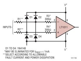
Figure 3. Limiting Fault Input Currents
