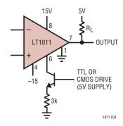
Figure 4. Typical Strobe Circuit
