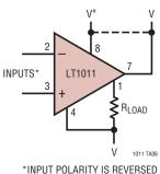
\*INPUT POLARITY IS REVERSED WHEN USING PIN 1 AS OUTPUT
