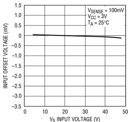
Figure 2.  $V_{OS}$  vs  $V_S$  Input Voltage
