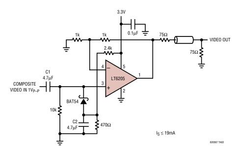
Figure 2. Clamped AC-Input Video Cable Driver
