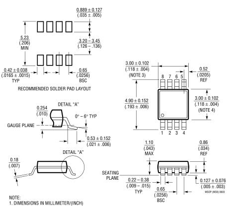
**MS8** Package 8-Lead Plastic MSOP (Reference LTC DWG # 05-08-1660)
