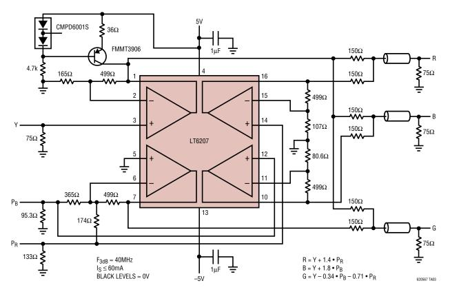
YP<sub>B</sub>P<sub>R</sub> to RGB Converter
