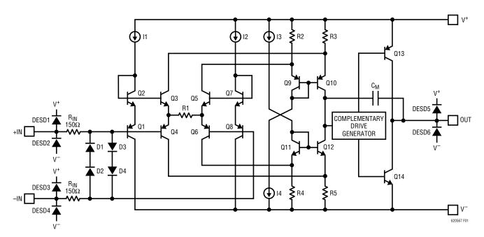
Figure 1. Simplified Schematic
