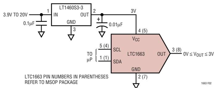
**Figure 2. LT1460 As Power Supply for the LTC1663**
