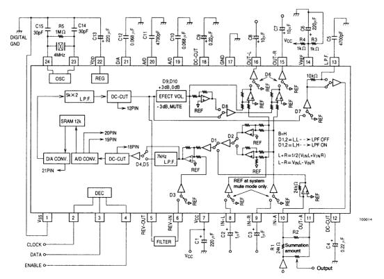
Note: The items D1 through D10 in the figure indicate points that are switched by the serial data.
