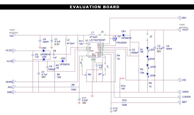
Figure 10 – LX1744EVAL Evaluation Board Schematic
