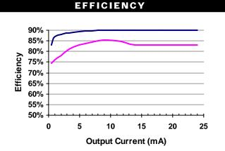
Figure 13 – LED Driver (Upper) and LCD Bias Efficiency  $V_{IN}$  = 5V, Four LEDs, L = 47 $\mu$ H, R<sub>CS</sub> = 4k $\Omega$   $V_{IN}$  = 3.6V, V<sub>OUT</sub> = 5.5V, L = 47 $\mu$ H
