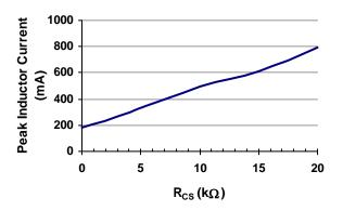
Figure 7 - Peak Current Programming Resistor
