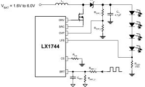
Figure 6 - LED Current Programming
