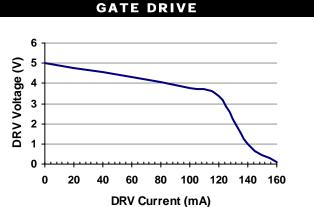
Figure 11 – Gate Drive Voltage Vs. Drive Current  $V_{IN}$  = 5V,  $T_A$  = 25°C
