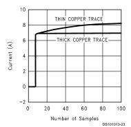
FIGURE 7. Transient Response to 7 Amp Step Current
