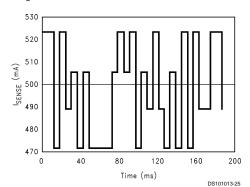
FIGURE 8. Typical Response of LM3814-1.0/LM3815-1.0
