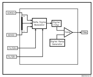
FIGURE 6. Functional block diagram of LM3814 and LM3815
