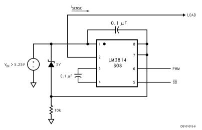
FIGURE 4. High Voltage Operation —  $\rm V_{IN}$  Greater Than 5.25V (High Side Sense) (PWM output is referred to Pin 7)
