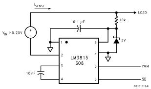
FIGURE 5. High Voltage Operation —  $\rm V_{IN}$  Greater Than 5.25V (Low Side Sense)
