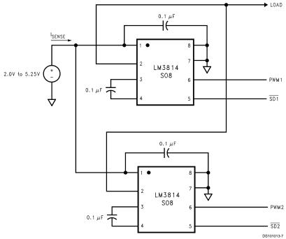
FIGURE 3. Paralleling LM3814 for Higher Load Current  $I_{TOTAL} = 2.2(D_1-0.5)I_{MAX} + 2.2(D_2-0.5)I_{MAX}$  where  $D_1$  is the duty cycle of PWM1 and  $D_2$  is the duty cycle of PWM2. Please refer to the Product Operation section for more information.
