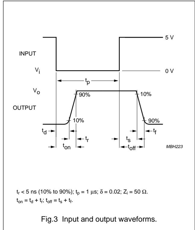
$t_r < 5 \text{ ns}$  (10% to 90%);  $t_p = 1 \mu\text{s}$ ;  $\delta = 0.02$ ;  $Z_i = 50 \Omega$ .
