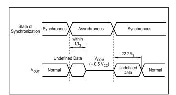
FIGURE 11. Loss of Synchronization and Analog Output State.
