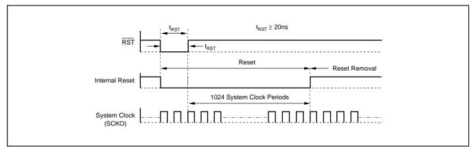
FIGURE 7. External Reset Operation.
