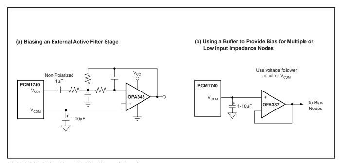
FIGURE 18. Using V<sub>COM</sub> To Bias External Circuitry.
