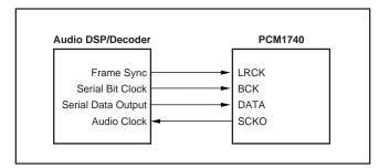
FIGURE 8. Interfacing the PCM1740 to an Audio DSP.
