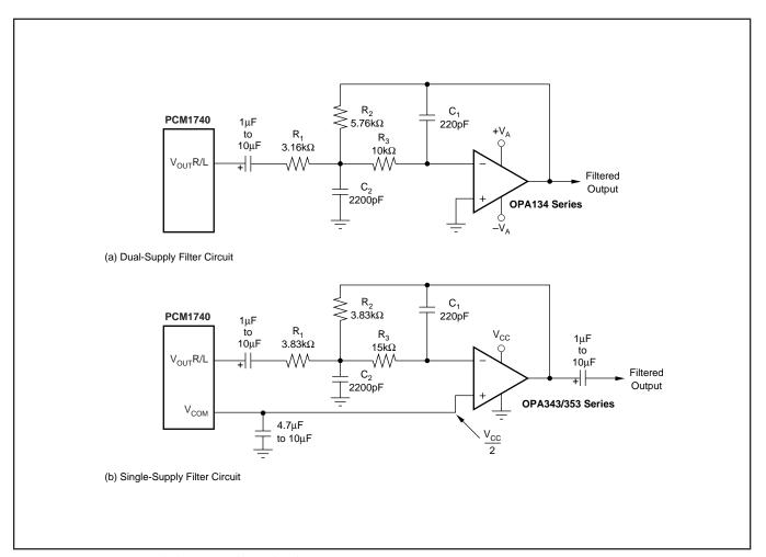
FIGURE 19. Recommended Output Filter Circuits.
