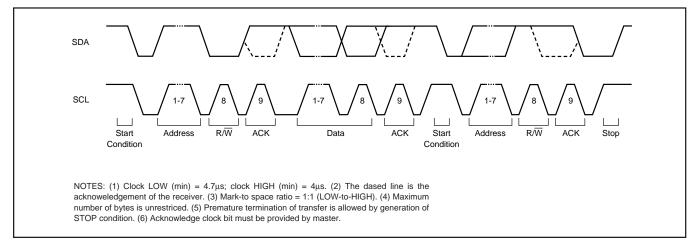
FIGURE 14. I<sup>2</sup>C Bus Data Transfer.
