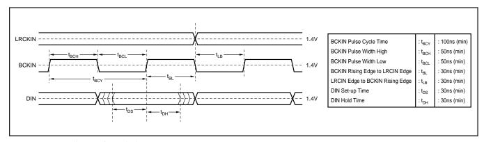
FIGURE 10. Audio Interface Timing.
