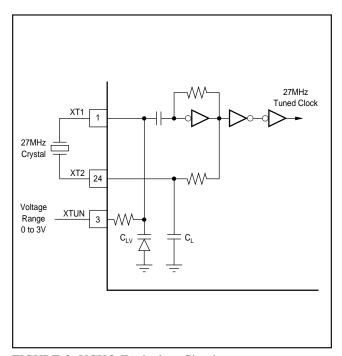
FIGURE 3. VCXO Equivalent Circuit.
