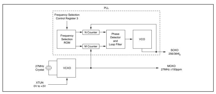
FIGURE 5. PLL Block Diagram.
