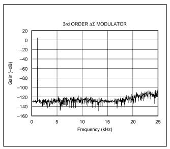
FIGURE 2. Quantization Noise Spectrum.
