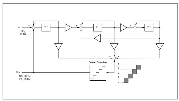
FIGURE 1. 5-Level  $\Delta\Sigma$  Modulator Block Diagram.
