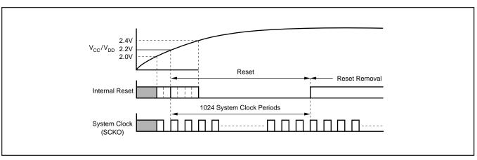
FIGURE 6. Power-On Reset Operation.
