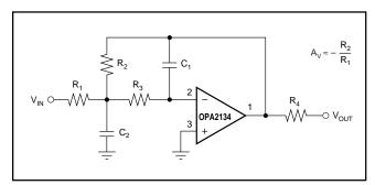
FIGURE 10. Dual-Supply Filter Circuit.
