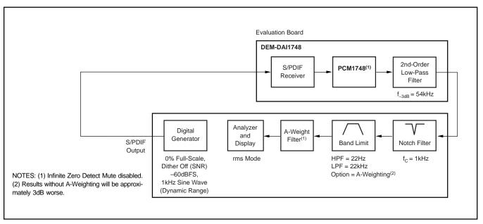
FIGURE 18. Test Setup for Dynamic Range and SNR Meeasurements.
