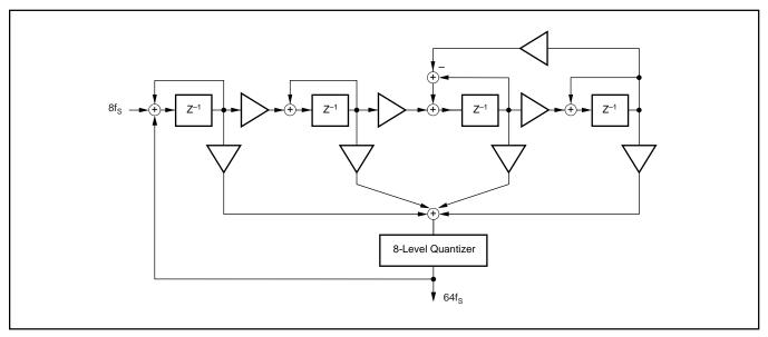
FIGURE 14. Eight-Level Delta-Sigma Modulator.
