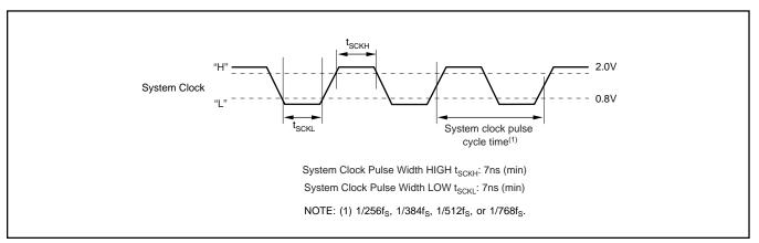
FIGURE 1. System Clock Input Timing.
