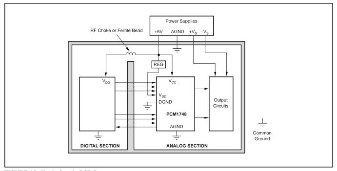
FIGURE 13. Single-Supply PCB Layout.
