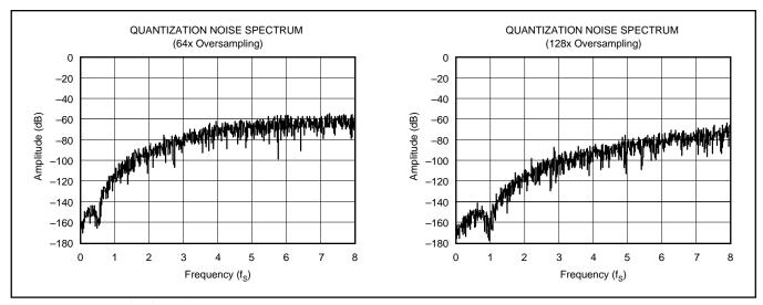
FIGURE 15. Quantization Noise Spectrum.
