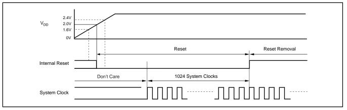
FIGURE 2. Power-On Reset Timing.
