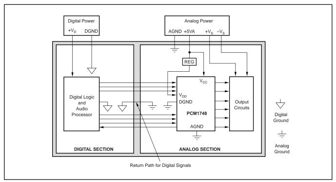
FIGURE 12. Recommended PCB Layout.
