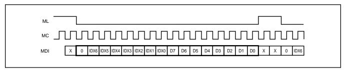
FIGURE 6. Register Write Operation.
