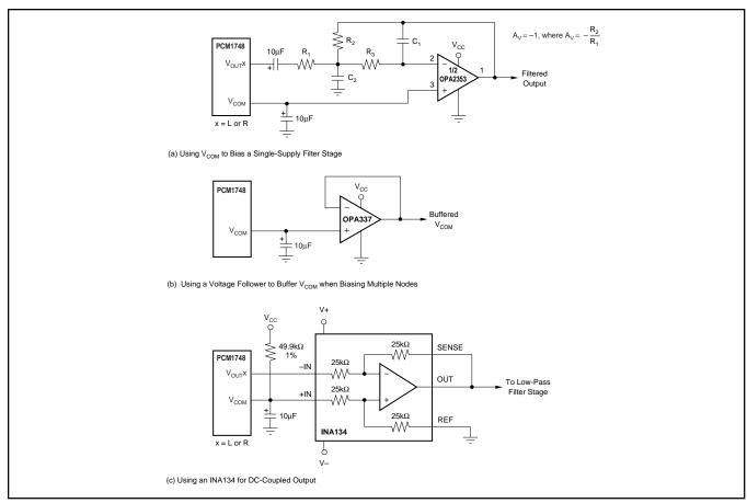
FIGURE 9. Biasing External Circuits Using the V<sub>COM</sub> Pin.
