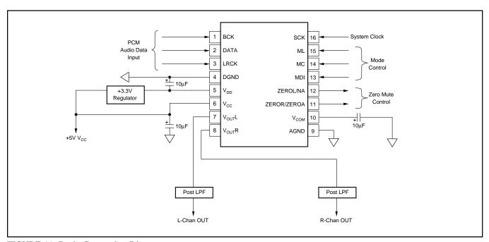
FIGURE 11. Basic Connection Diagram.
