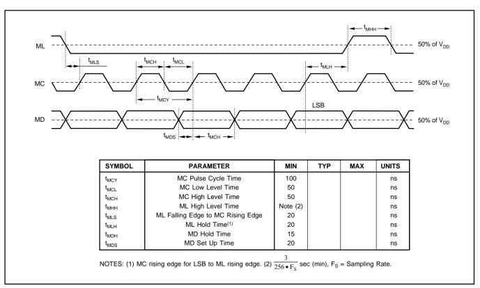
FIGURE 7. Control Interface Timing.
