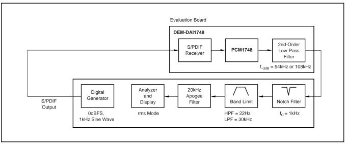
FIGURE 17. Test Setup for THD+N Measurements.
