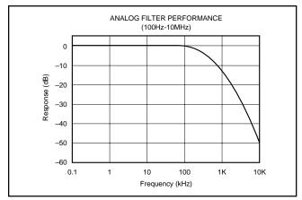
FIGURE 8. Output Filter Frequency Response.
