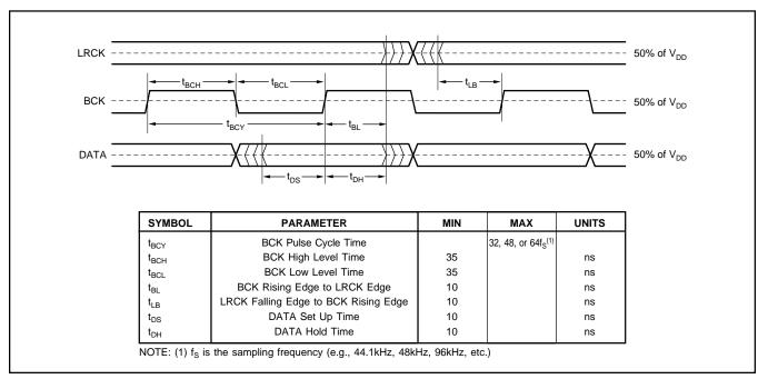
FIGURE 4. Audio Interface Timing.
