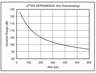
FIGURE 16. Jitter Sensitivity.
