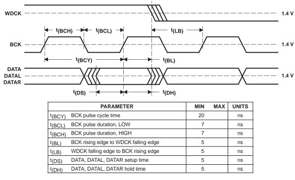
Figure 41. Audio Interface Timing for External Digital Filter (Internal DF Bypass Mode) Application
