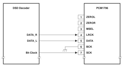
Figure 42. Connection Diagram in DSD Mode
