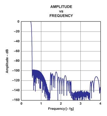
Figure 1. Frequency Response, Sharp Rolloff
