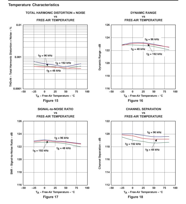
NOTE: PCM mode,  $V_{DD}$  = 3.3 V,  $V_{CC}$  = 5 V, measurement circuit is Figure 36.
