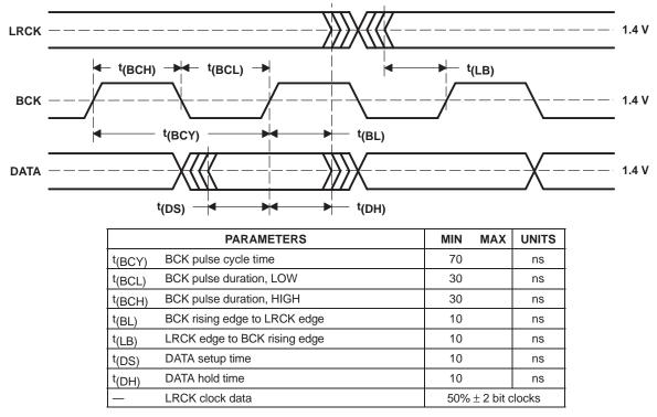
Figure 26. Timing of Audio Interface
