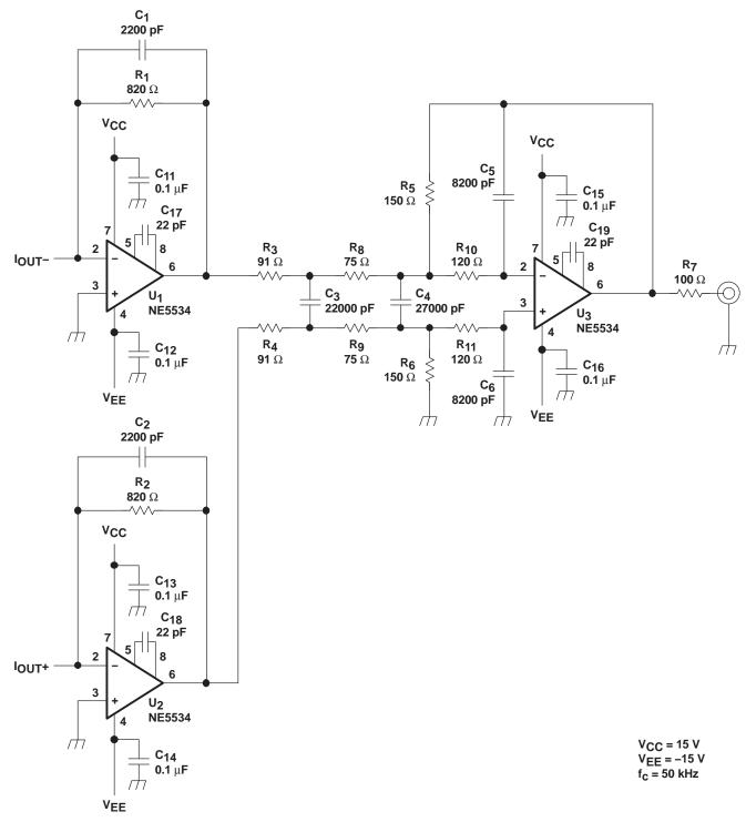
Figure 37. Measurement Circuit for DSD
