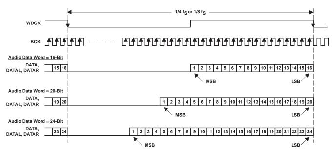
Figure 40. Audio Data Input Format for External Digital Filter (Internal DF Bypass Mode) Application
