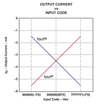
Figure 64. The Relationship Between Digital Input and Analog Output
