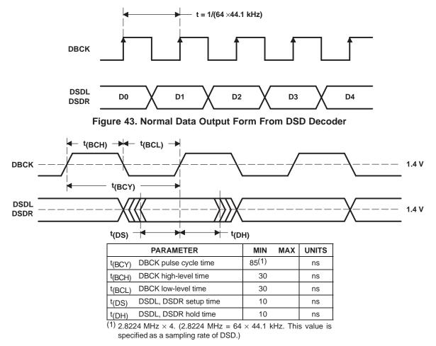
Figure 44. Timing for DSD Audio Interface
