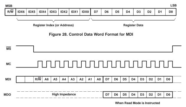
NOTE: Bit 15 is used for selection of write or read. Setting R/W = 0 indicates a write, while R/W = 1 indicates a read. Bits 14–8 are used for the register address. Bits 7–0 are used for register data.
