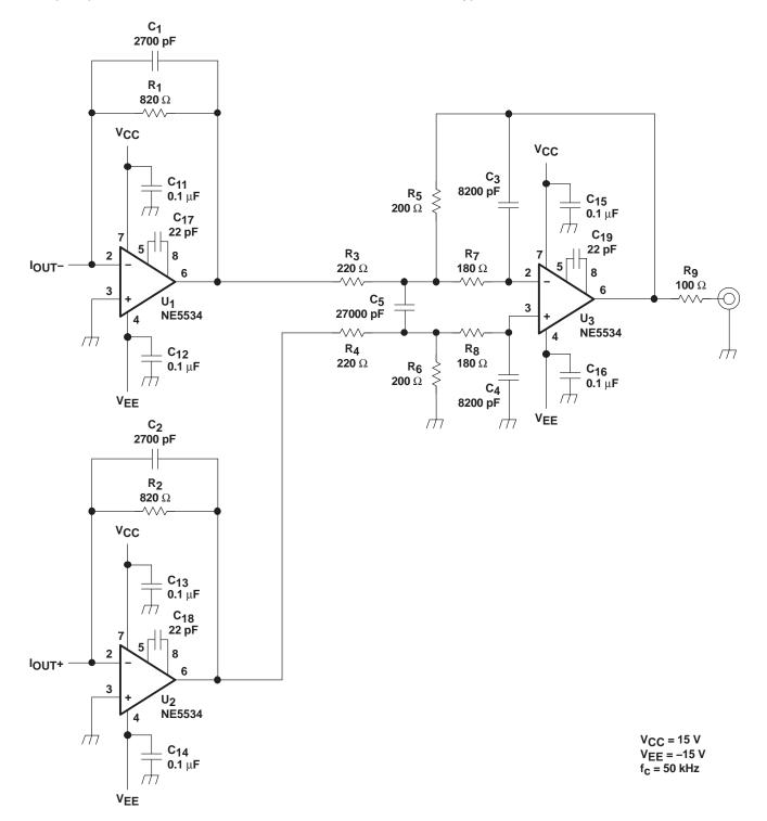
Figure 36. Measurement Circuit for PCM
