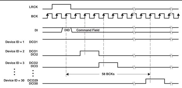
Figure 56. Device ID Determination Sequence
