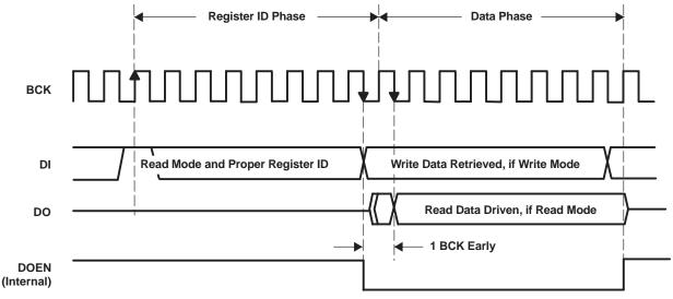
Figure 59. TDMCA Write and Read Operation Timing
