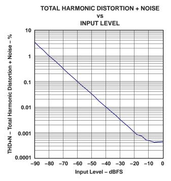
NOTE: PCM mode, f<sub>S</sub> = 48 kHz, T<sub>A</sub> = 25°C, V<sub>DD</sub> = 3.3 V, V<sub>CC</sub> = 5 V, NOTE: DSD mode (FIR-2), 32768 point 8 average, T<sub>A</sub> = 25°C, measurement circuit is Figure 36.
