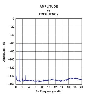
$V_{DD}$  = 3.3 V,  $V_{CC}$  = 5 V, measurement circuit is Figure 37.
