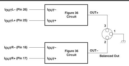
Figure 38. Measurement Circuit for Monaural Mode
