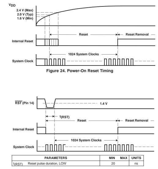
Figure 25. External Reset Timing
