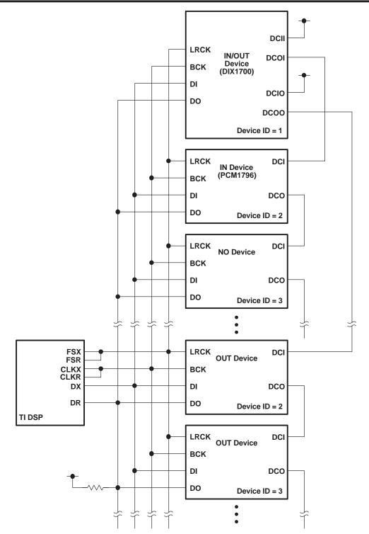
Figure 55. IN Daisy Chain and OUT Daisy Chain Connection for a Multichip System
