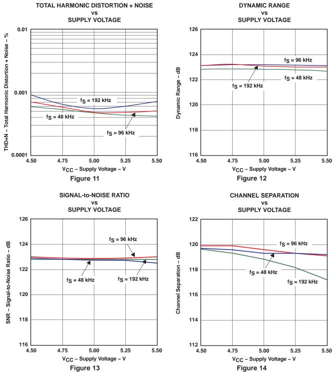
NOTE: PCM mode,  $T_A = 25^{\circ}C$ ,  $V_{DD} = 3.3$  V, measurement circuit is Figure 36.
