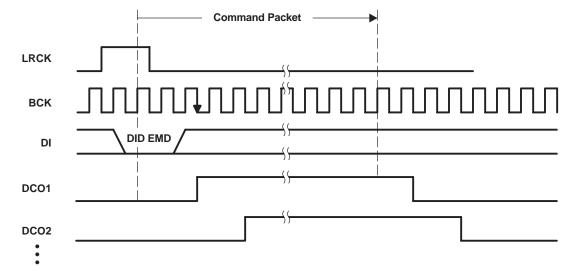
Figure 62. DCO Output Timing With Skip Operation (for Command Packet 1)
