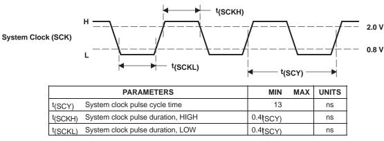
Figure 23. System Clock Input Timing
