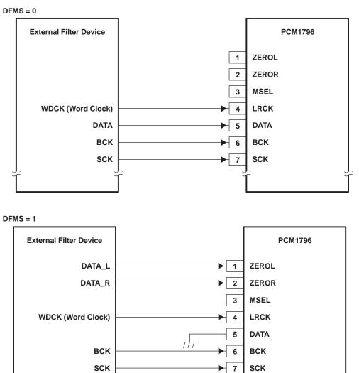
Figure 39. Connection Diagram for External DIgital Filter (Internal DF Bypass Mode) Application
