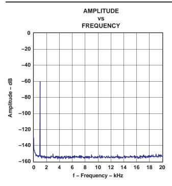
NOTE: PCM mode,  $f_S = 48 \text{ kHz}$ , 32768 point 8 average,  $T_A = 25^{\circ}C$ ,  $V_{DD} = 3.3 \text{ V} \text{ V}_{CC} = 5 \text{ V}$ , measurement circuit is Figure 36.
