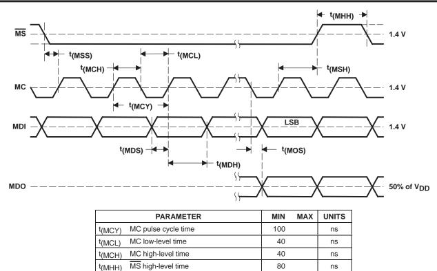
Figure 30. Control Interface Timing
