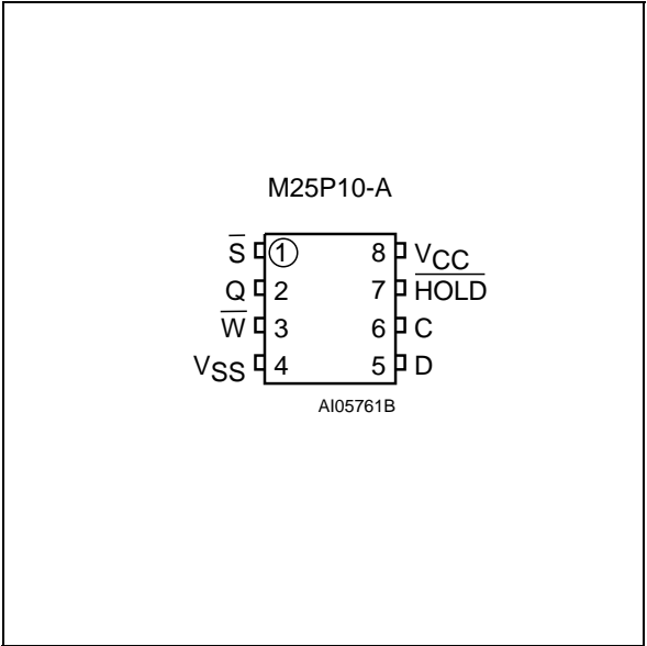
Figure 3. SO and VFQFPN Connections
