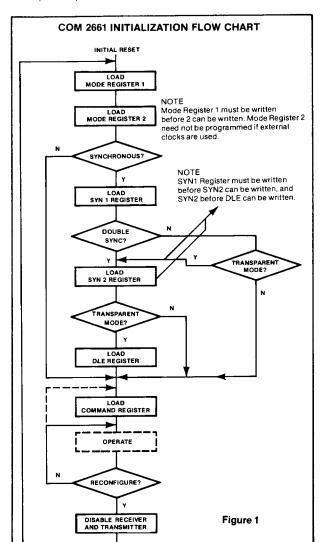
than the required number of accesses are made, the internal sequencer recycles to point at the first register. The pointers are reset to SYN1 Register and Mode Register 1 by a RESET input or by performing a "Read Command Register" operation, but are unaffected by any other read or write operation.
