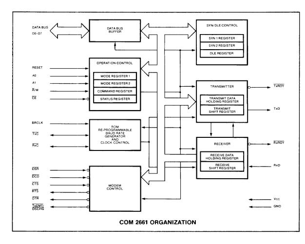
The COM 2661 is organized into 6 major sections. Communication between each section is achieved via an internal data and control bus. The data bus buffer allows a processor access to all internal registers on the COM 2661. The differences between the COM 2661 and COM 2651 are outlined in table 1.
