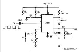
$V_{OUT} = f_{IN} \times 2.09V \times \frac{R_L}{R_S} \times (R_t C_t)$
