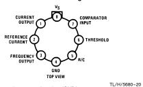
Note: Metal case is connected to pin 4 (GND.)
