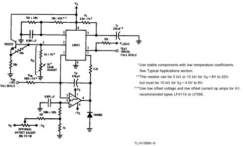
FIGURE 4. Precision Voltage-to-Frequency Converter, 100 kHz Full-Scale, ± 0.03% Non-Linearity
