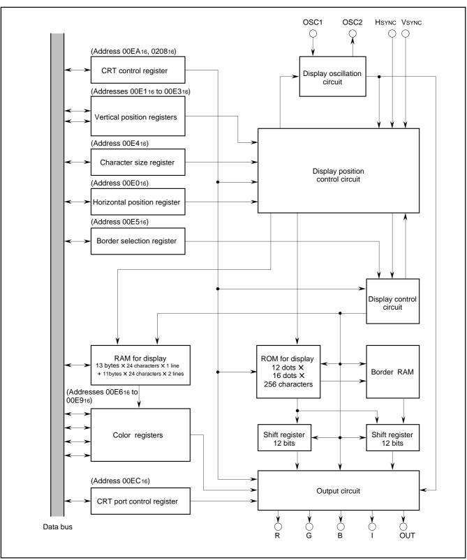
Fig. 45. Block Diagram of CRT Display Circuit
