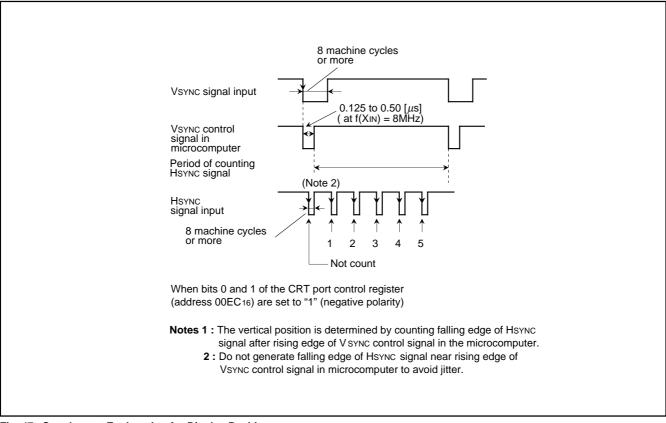
Fig. 47. Supplement Explanation for Display Position
