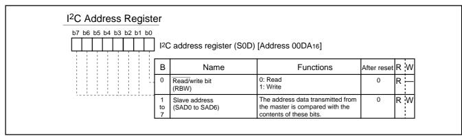
Fig. 25. I<sup>2</sup>C Address Register
