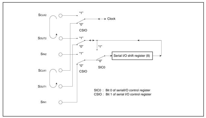
Fig. 22. Signals on Serial I/O Common Transmission/Reception Mode
