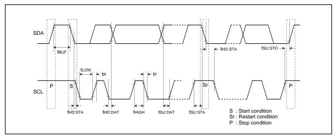
Fig. 83. Definition diagram of timing on multi-master I<sup>2</sup>C-BUS
