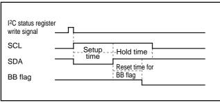
Fig. 32. STOP Condition Generation Timing Diagram
