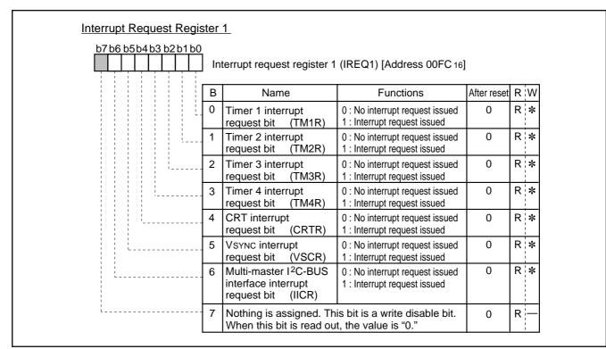
Fig. 10. Interrupt Request Register 1
