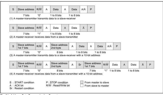
Fig. 34. Address Data Communication Format
