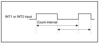
Fig. 71. Measuring Interval
