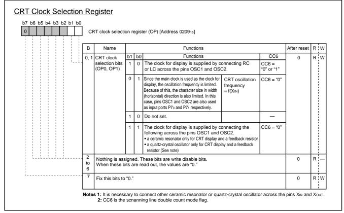
Fig. 68. CRT Clock Selection Register
