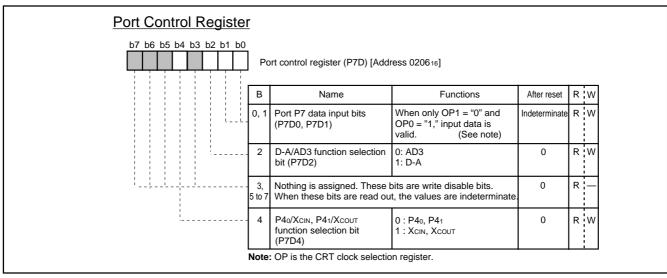
Fig. 65. Port Control Register
