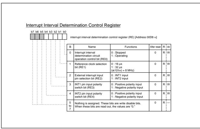
Fig. 70. Interrupt Interval Determination Control Register
