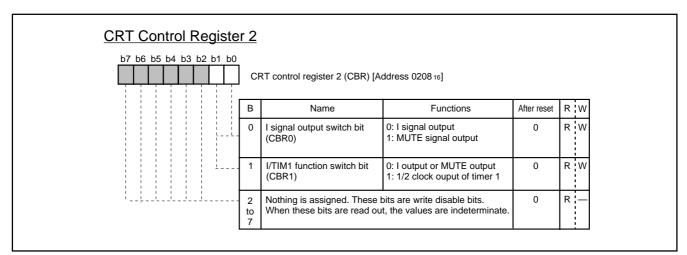
Fig. 67. CRT Control Register 2
