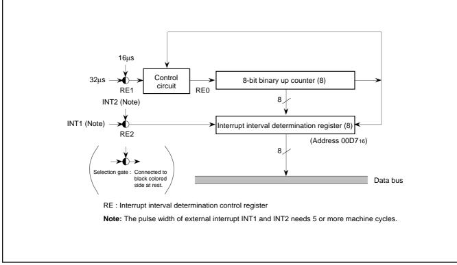
Fig. 69. Block Diagram of Interrupt Interval Determination Circuit
