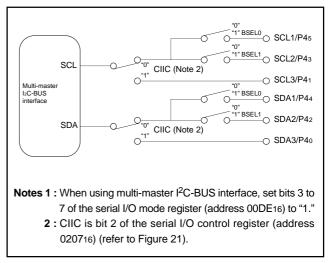
Fig. 27. Connection Port Control by BSEL0 and BSEL1
