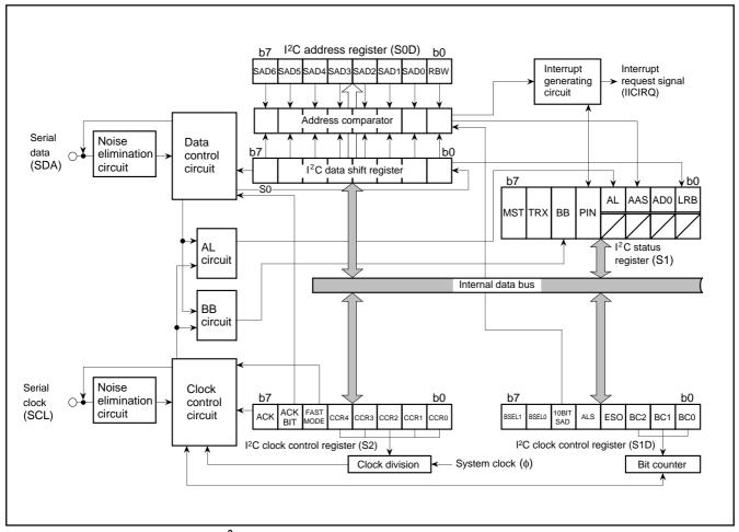
Fig. 23. Block Diagram of Multi-master I<sup>2</sup>C-BUS Interface
