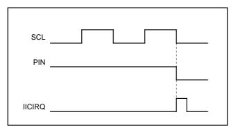
Fig. 30. Interrupt Request Signal Generation Timing
