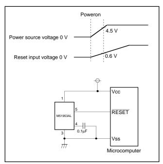
Fig. 74. Example of Reset Circuit
