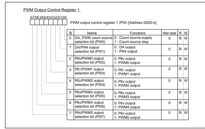
Fig. 38. PWM Output Control Register 1
