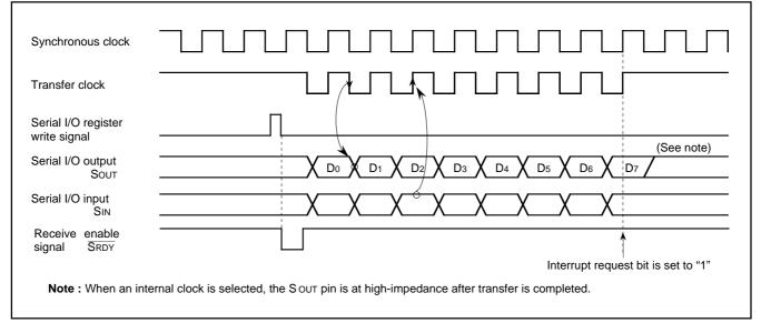
Fig. 19. Serial I/O Timing (for LSB first)
