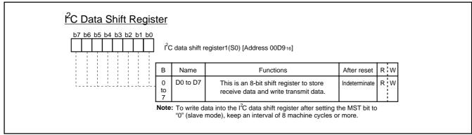
Fig. 24. I<sup>2</sup>C Data Shift Register
