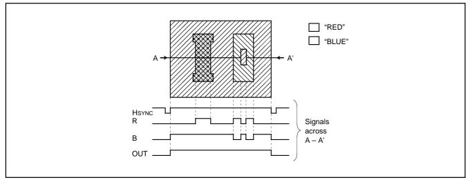
Fig. 66. Example of Raster Coloring
