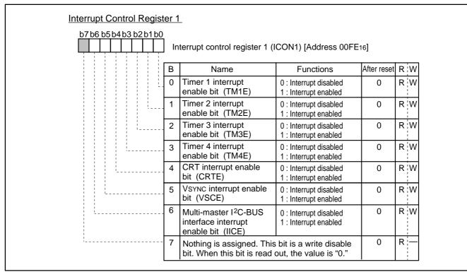
Fig. 12. Interrupt Control Register 1
