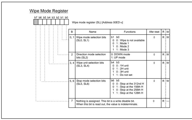
Fig. 63. Structure of Wipe Mode Register
