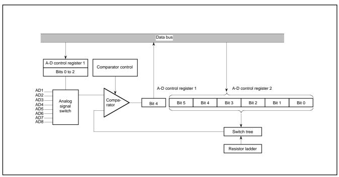
Fig. 40. A-D Comparator Block Diagram
