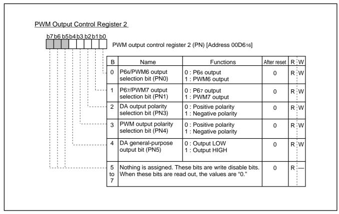
Fig. 39. PWM Output Control Register 2
