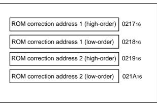
Fig. 72. ROM Correction Address Registers
