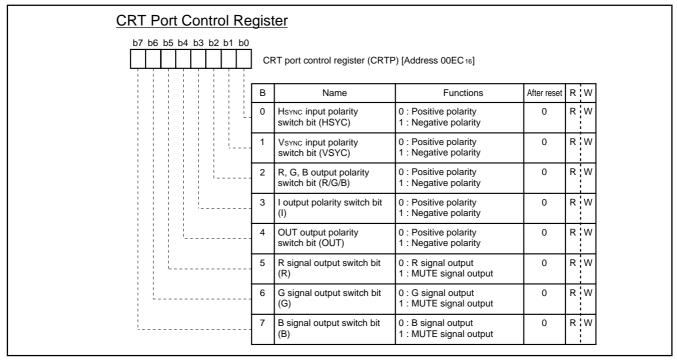
Fig. 64. CRT Port Control Register
