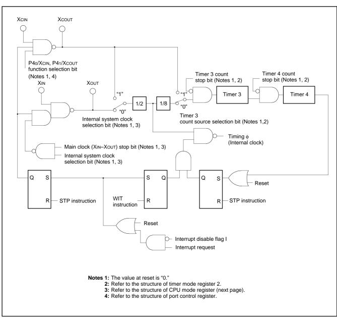
Fig. 78. Clock Generating Circuit Block Diagram
