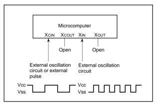
Fig. 77. External Clock Input Circuit Example
