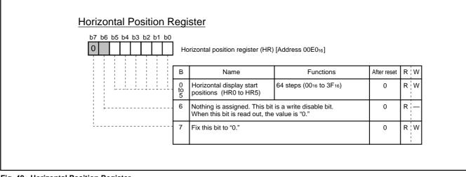
Fig. 49. Horizontal Position Register
