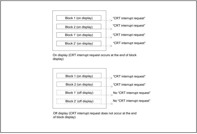
Fig. 59. Timing of CRT Interrupt Request
