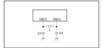
Fig. 80. Display Oscillation Circuit
