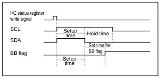
Fig. 31. START Condition Generation Timing Diagram
