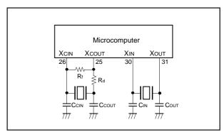
Fig. 76. Ceramic Resonator Circuit Example
