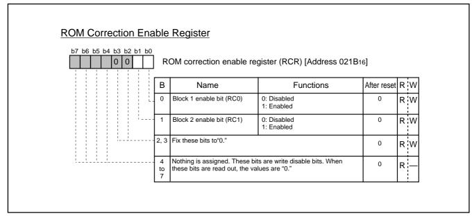
Fig. 73. ROM Correction Enable Register
