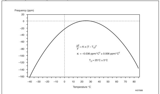
Figure 17. Crystal accuracy across temperature
