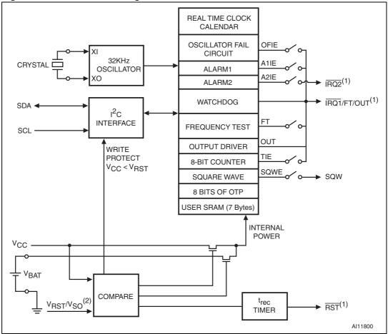
Figure 8. M41T83 block diagram
