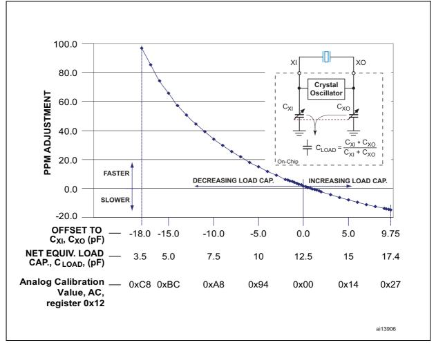
Figure 18. Clock accuracy vs. on-chip load capacitance
