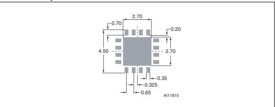
Note: Dimensions are shown in millimeters (mm).
