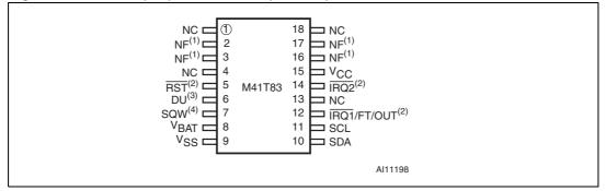
1. NF pins must be tied to  $V_{\mbox{SS}}.$  Pins 2 and 3, and 16 and 17 are internally shorted together.
