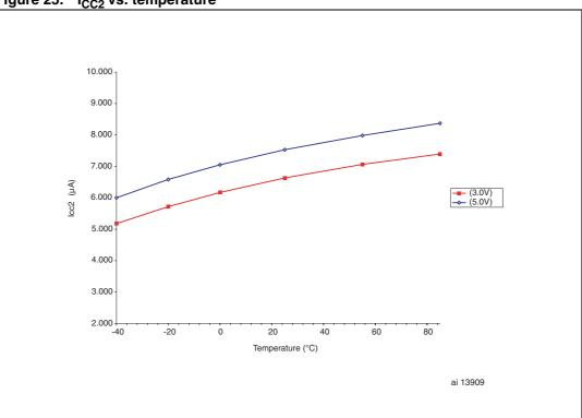
Figure 25. I<sub>CC2</sub> vs. temperature
