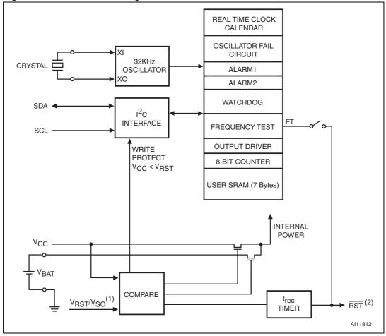
Figure 6. M41T82 block diagram
