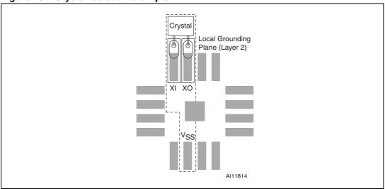
Figure 20. Crystal isolation example
