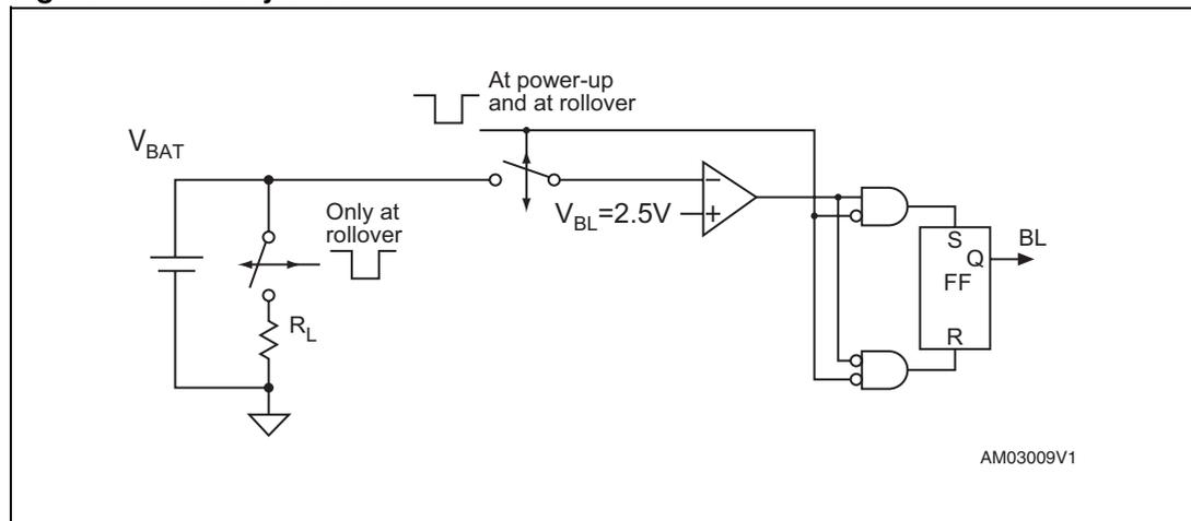
The M41T8x only checks the battery when powered by  $V_{CC}$ . It does not check the battery while in backup mode. Thus, users are advised that during long periods in backup mode, the battery can drop to a level at which timekeeping may fail or data becomes corrupted. If, at power-up, a battery low is indicated, data integrity should be verified.
