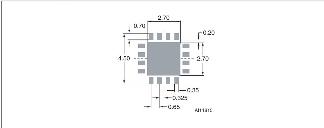
*Note: Dimensions are shown in millimeters (mm).*
