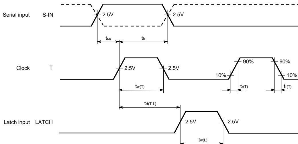
**SWITCHING CHARACTERISTICS** ( $T_a = 25^\circ\text{C}$ ,  $V_{CC} = 5\text{V}$ , unless otherwise noted)
