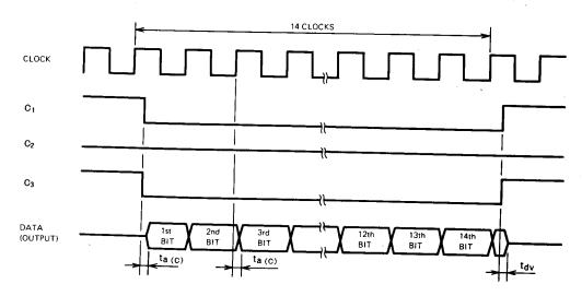
The 1st bit of output data is output after access time of  $t_{a(C)}$  from the mode control transition. And other bits are output after  $t_{a(C)}$  from positive edge of clock.
