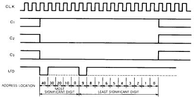
Note 3: The address is designated by one-of-tive and one-of-ten coded digits. The figure shows designation of the address: 49.
