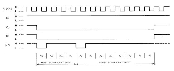
Note 2: The addresses from  $A_{00}$  to  $A_{37}$  are designated by one-of-four and one-of-eight coded digits. The above figure shows designation of address  $A_{37}$
