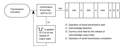
(2) The writing operation of the setting data (FFh, 80h, EEh) into M65667SP internal address of 04h to 06h
