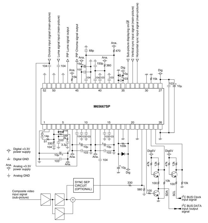
Separate Y/C signals by using LC-tank circuit or LPF,BPF for Y/C signals level adjust. And then mix both signals for sub-picture input video signal.
