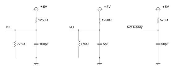
Fig 1. I/O Output Load
