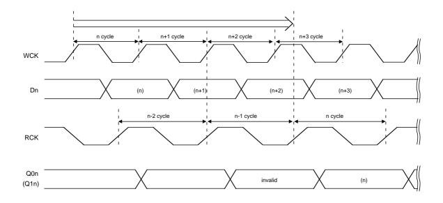
• Reading longest n-cycle write data "n": 1 line delay
