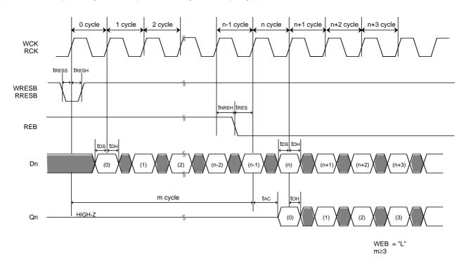
• Reading shortest n-cycle write data "n" (Reading side n-1 cycle starts after the end of writing side n-1 cycle.)
