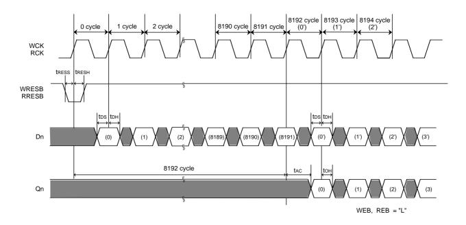
• n-bit delay bit (Reset at cycles according to the delay length)
