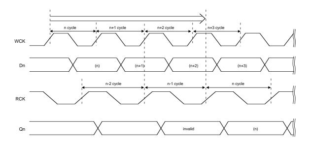
• Reading longest n-cycle write data "n": 1 line delay (When writing side n-cycle <2>\* starts, reading side n cycle <1>\* then starts.)
