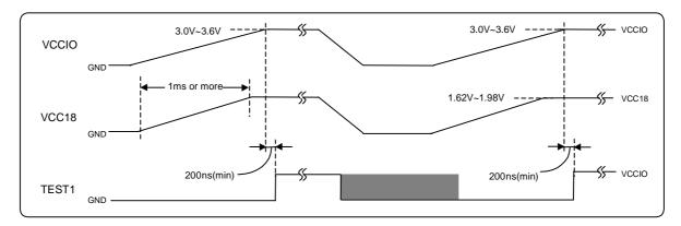
Note: Some circuits of internal FIFO can be initialized by the TEST1 pin even if the power-on time of the Vcc18 is 1 msec or less.
