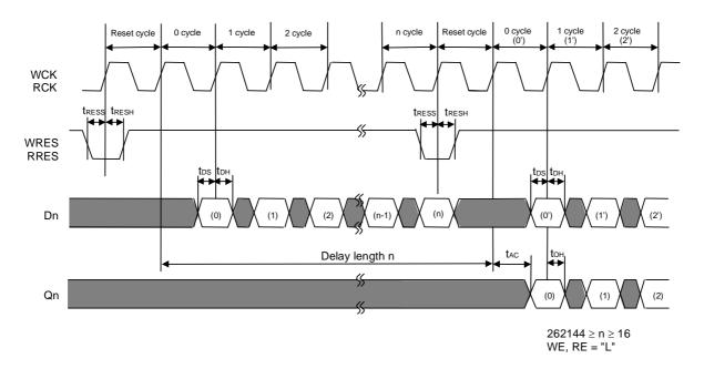
Note: The intervals of 16 cycles or more between a write cycle and a read cycle should be secured to read data written in a certain cycle.
