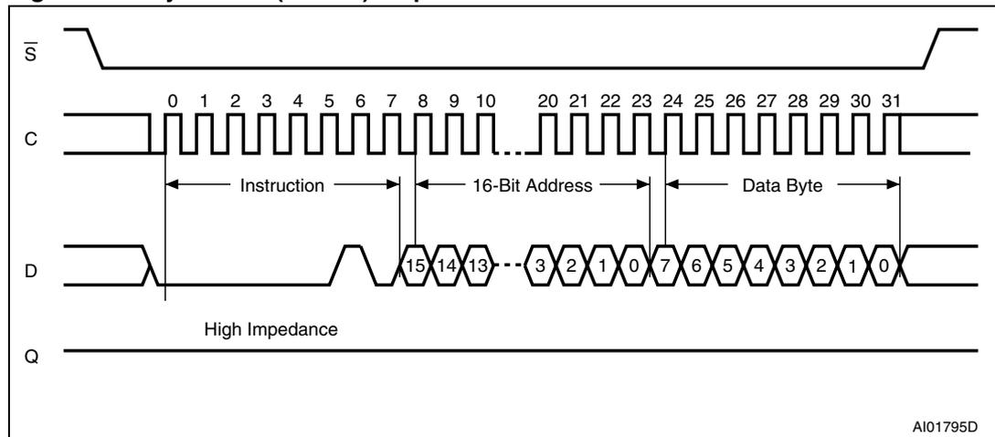
1. Depending on the memory size, as shown in [Table 7.](#), the most significant address bits are Don't Care.
