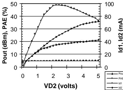
Output Power, Drain Currents and Efficiency vs.  $V_{DD1}$  for Power Control  $P_{IN} = 0\text{ dBm}$ ,  $f_c = 2450\text{ MHz}$ ,  $V_{DD2} = 3\text{ V}$
