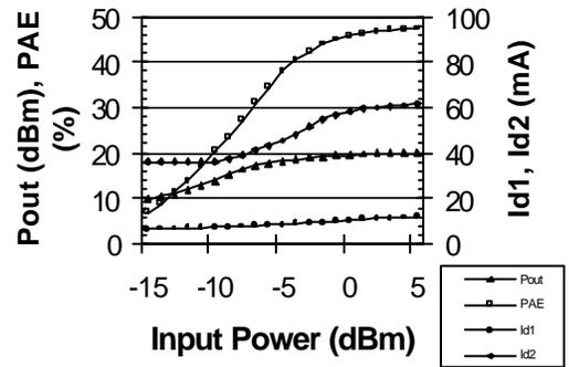
Output Power, Drain Currents and Efficiency vs. Supply Voltage  $P_{IN} = 0\text{ dBm}$ ,  $f_c = 2450\text{ MHz}$ ,  $V_{DD1} = 2.5\text{ V}$
