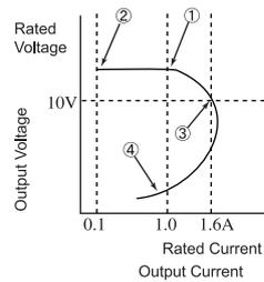
Fig2. Output Voltage/Current
