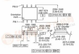
8- Lead SOP outline dimensions Narrow body .150 (All dimensions per JEDEC No. MS-012-AA, Issue C) Dimensions in ( ) are in mm.
