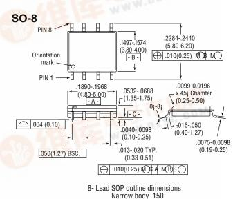
Narrow body .150 (All dimensions per JEDEC No. MS-012-AA, Issue C) Dimensions in () are in mm.
