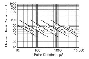
Fig. 2E. Maximum Peak Current vs. Pulse Duration
