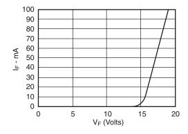
Fig. 3B. Forward Current vs. Forward Voltage
