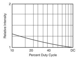
Fig. 3E. Relative Luminous Intensity vs. Duty Cycle
