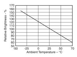
Fig. 3C. Relative Luminous Intensity vs. Temperature (See Note 2)
