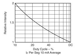
Fig. 4E. Relative Luminous Intensity vs. Duty Cycle
