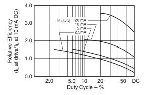
Fig. 2D. Relative Efficiency vs. Duty Cycle
