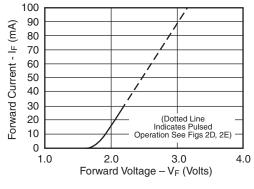
Fig. 2B. Forward Current vs.Forward Voltage
