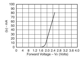
Fig. 4B. Forward Current vs. Forward Voltage
