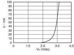
Fig. 1B. Forward Current vs. Forward Voltage
