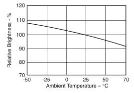
Fig. 1C. Relative Luminous Intensity vs. Temperature (See Note 2)
