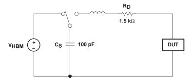
Figure 5. HBM ESD Test Circuit
