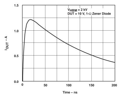
Figure 6. Typical HBM Current Waveform
