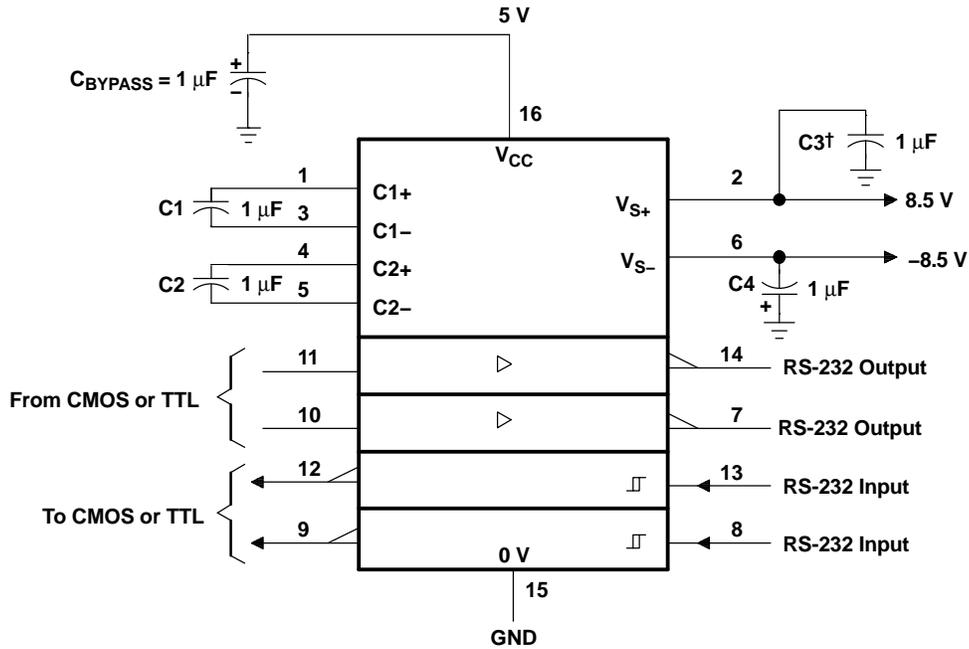
† C<sub>3</sub> can be connected to V<sub>CC</sub> or GND.
