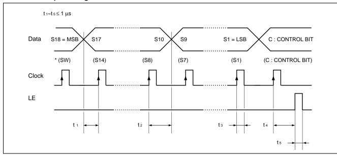
Notes: Paranthesis data is used for setting divide ratio of programmable reference divider.
