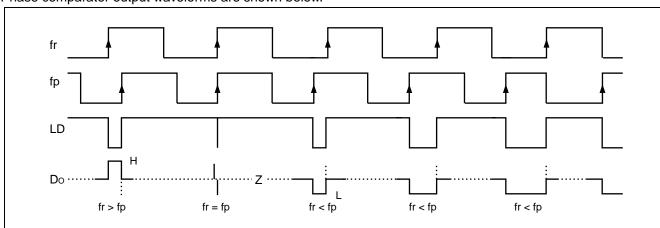
Phase comparator output waveforms are shown below.
