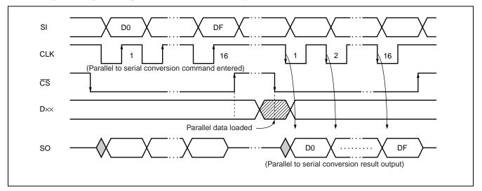
• I/O Expander Operation (parallel to serial conversion)
