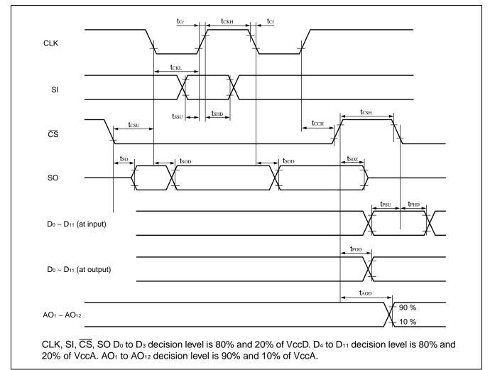
• Input/Output Timing (CS method)
