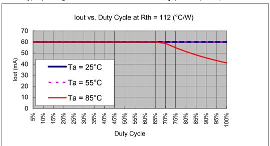
The maximum power dissipation,  $P_D(max) = (Tj-Ta) / R_{th(j-a)}$ , decreases as the ambient temperature increases.
