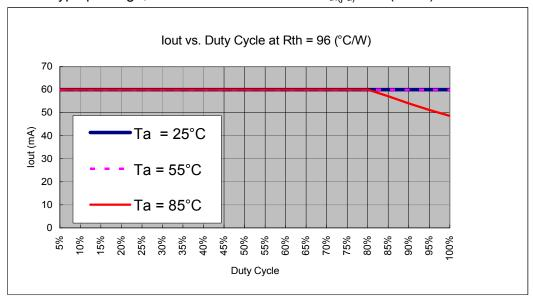
For CP type package, the thermal resistance is  $R_{th(j-a)}$  = 112 (°C/W)
