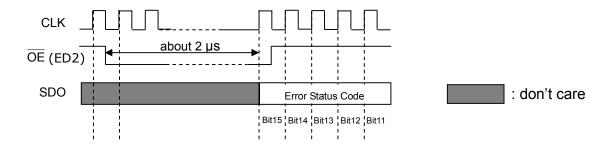
A system controller can read Error Status codes through SDO pin.
