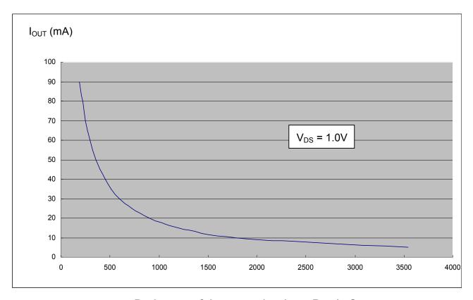
Resistance of the external resistor,  $R_{\text{ext}}$ , in  $\Omega$
