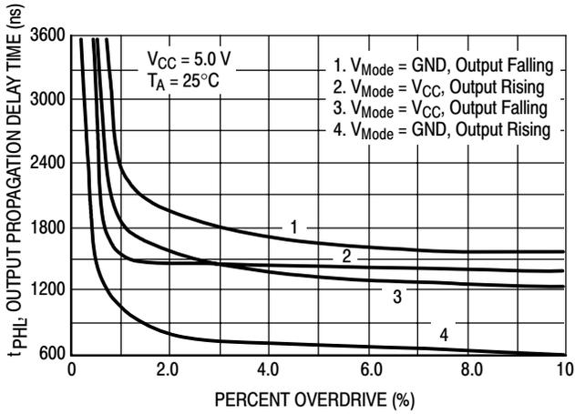
Figure 4. Output Propagation Delay Time versus Percent Overdrive
