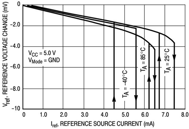
Figure 10. Reference Voltage Change versus Source Current
