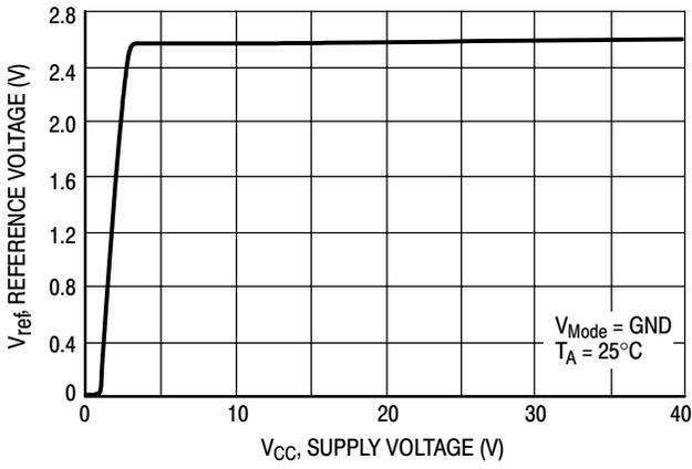
Figure 8. Reference Voltage versus Supply Voltage
