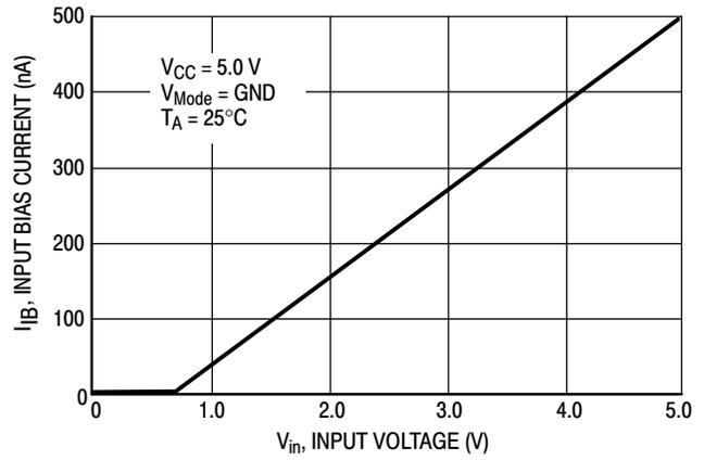
Figure 3. Comparator Input Bias Current versus Input Voltage
