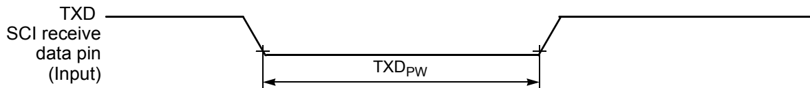
Figure 10-16 TXD Pulse Width
