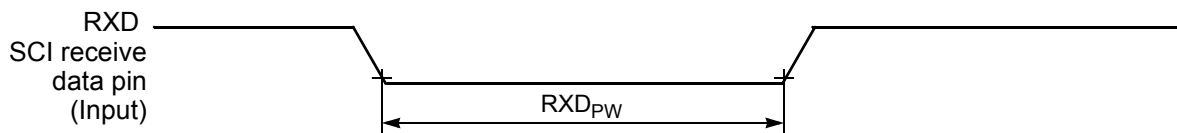
Figure 10-15 RXD Pulse Width
