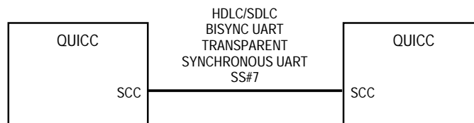
Figure 1-15. Multiple QUICC Point-to-Point Implementation
