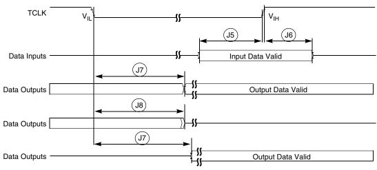
Figure 15. Boundary Scan (JTAG) Timing
