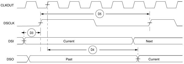
Figure 19. BDM Serial Port AC Timing
