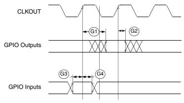
Figure 6. GPIO Timing
