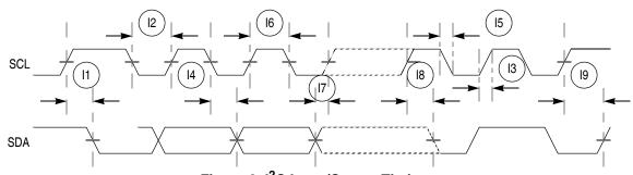
Figure 8. I<sup>2</sup>C Input/Output Timings
