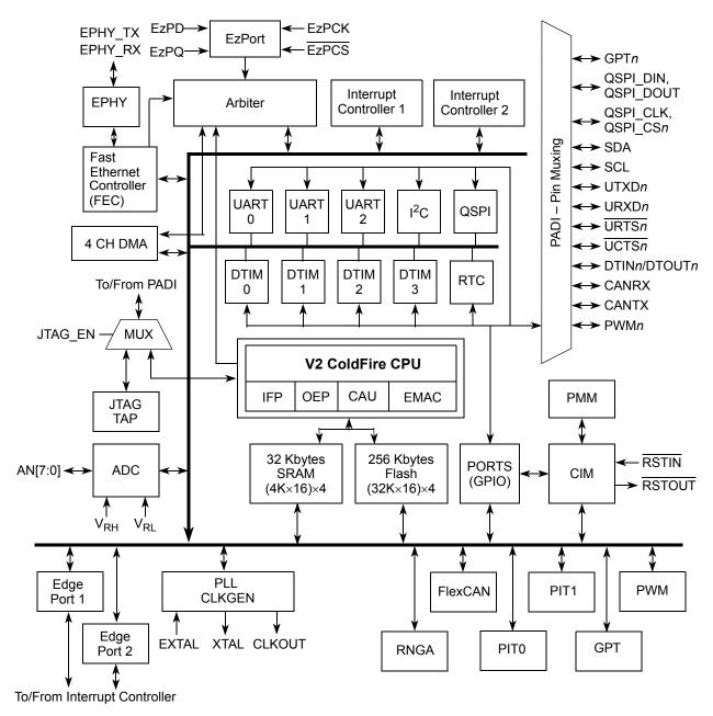
Figure 1. MCF52235 Block Diagram
