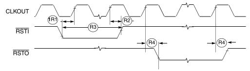
Figure 7. RSTI and Configuration Override Timing
