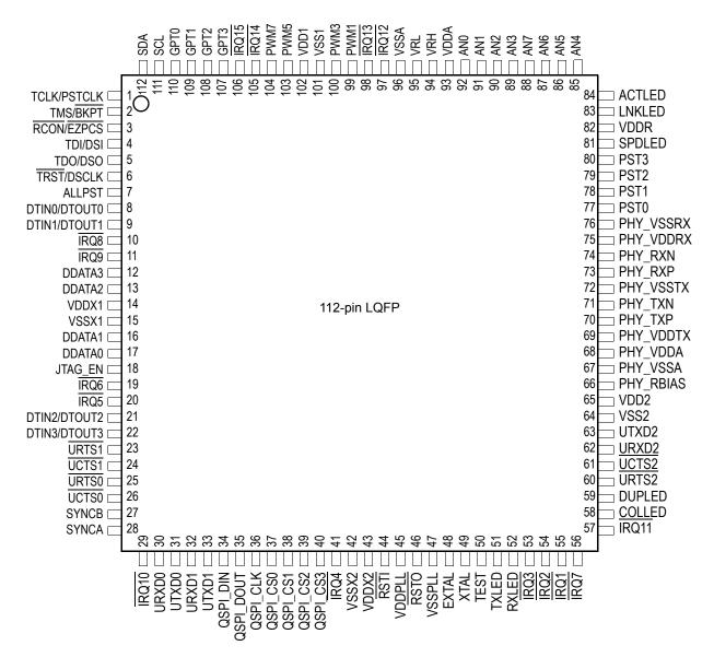
Figure 3. 112-pin LQFP Pin Assignments
