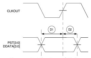
Figure 18. Real-Time Trace AC Timing
