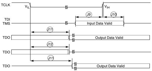
**Figure 16. Test Access Port Timing**
