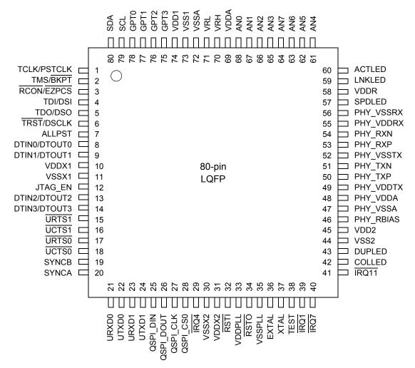
Figure 2. 80-pin LQFP Pin Assignments
