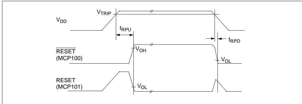
FIGURE 1-1: MCP100/101 Timing Diagram
