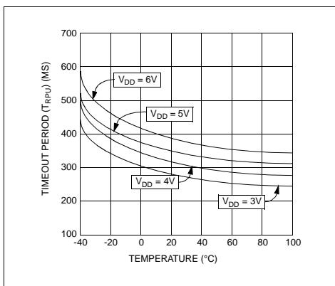
FIGURE 2-3: Typical  $t_{RPU}$  vs. Temperature
