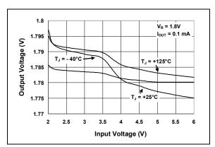
**FIGURE 2-5:** Output Voltage vs. Input Voltage  $(V_R = 1.8V)$ .
