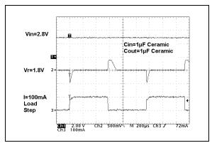
**FIGURE 2-18:** Dynamic Load Step  $(V_R = 1.8V)$ .
