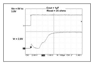
**FIGURE 2-26:** Start-up From  $V_{IN}$   $(V_R = 2.8V)$ .
