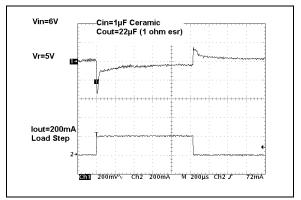
**FIGURE 2-22:** Dynamic Load Step  $(V_R = 5.0V)$ .
