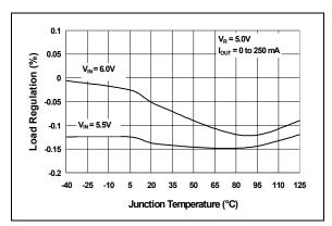
**FIGURE 2-29:** Load Regulation vs. Junction Temperature ( $V_R = 5.0V$ ).
