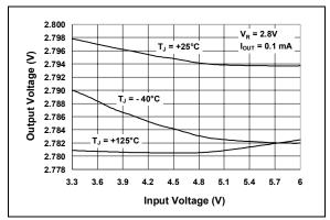
**FIGURE 2-6:** Output Voltage vs. Input Voltage  $(V_R = 2.8V)$ .
