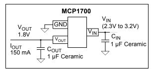
FIGURE 6-1: Typical Application Circuit.
