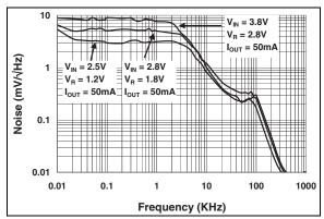
FIGURE 2-16: Noise vs. Frequency.
