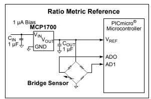
FIGURE 6-2: Using the MCP1700 as a voltage reference.
