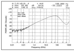
**FIGURE 2-15:** Power Supply Ripple Rejection vs. Frequency ( $V_R = 2.8V$ ).
