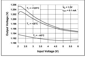
**FIGURE 2-4:** Output Voltage vs. Input Voltage  $(V_R = 1.2V)$ .
