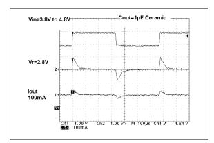
**FIGURE 2-23:** Dynamic Line Step  $(V_R = 2.8V)$ .
