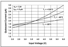
FIGURE 2-1: Input Quiescent Current vs. Input Voltage.
