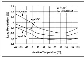
**FIGURE 2-27:** Load Regulation vs. Junction Temperature ( $V_R = 1.8V$ ).
