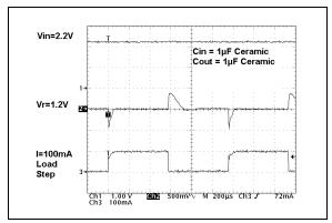
**FIGURE 2-17:** Dynamic Load Step  $(V_R = 1.2V)$ .
