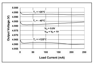
**FIGURE 2-11:** Output Voltage vs. Load Current ( $V_R = 5.0V$ ).
