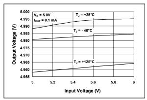
**FIGURE 2-7:** Output Voltage vs. Input Voltage  $(V_R = 5.0V)$ .
