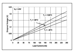
**FIGURE 2-12:** Dropout Voltage vs. Load Current ( $V_R = 2.8V$ ).
