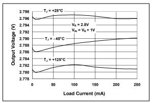
**FIGURE 2-10:** Output Voltage vs. Load Current ( $V_R = 2.8V$ ).
