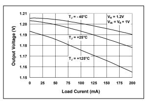
**FIGURE 2-8:** Output Voltage vs. Load Current ( $V_R = 1.2V$ ).
