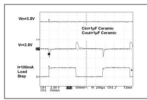
**FIGURE 2-19:** Dynamic Load Step  $(V_R = 2.8V)$ .
