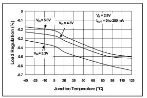
**FIGURE 2-28:** Load Regulation vs. Junction Temperature ( $V_R = 2.8V$ ).
