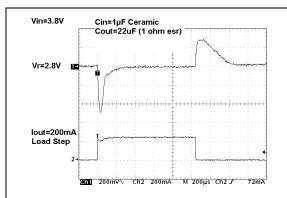
FIGURE 2-21: Dynamic Load Step  $(V_R = 2.8V)$ .
