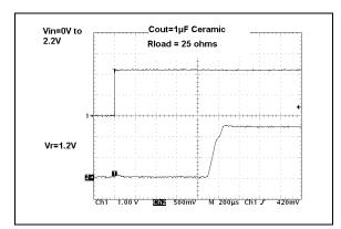
**FIGURE 2-24:** Startup From  $V_{IN}$   $(V_R = 1.2V)$ .
