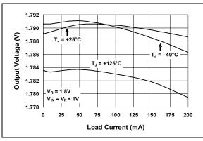
**FIGURE 2-9:** Output Voltage vs. Load Current ( $V_R = 1.8V$ ).
