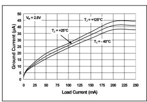
FIGURE 2-2: Ground Current vs. Load Current.
