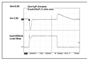
**FIGURE 2-20:** Dynamic Load Step  $(V_R = 1.8V)$ .
