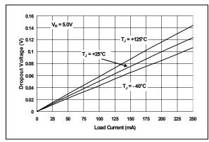
**FIGURE 2-13:** Dropout Voltage vs. Load Current ( $V_R = 5.0V$ ).
