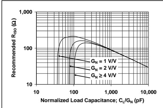
**FIGURE 4-4:** Recommended  $R_{ISO}$  Values for Capacitive Loads.
