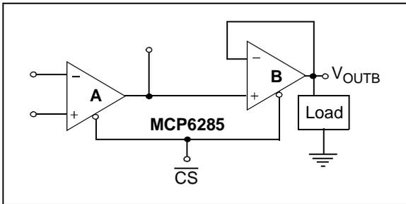
**FIGURE 4-9:** Isolating the Load with a Buffer.
