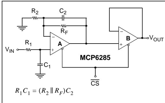
**FIGURE 4-12:** Buffered Non-inverting Integrator with Chip Select.
