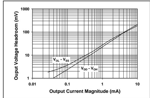
**FIGURE 2-16:** Output Voltage Headroom vs. Output Current Magnitude.
