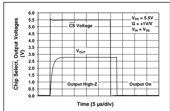
**FIGURE 2-30:**  $\overline{\text{CS}}$  to Amplifier Output Response Time at  $V_{DD} = 5.5\text{V}$  (MCP6283 and MCP6285 only).
