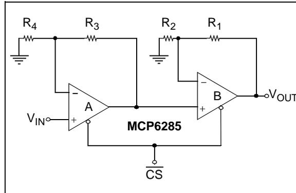
**FIGURE 4-10:** Cascaded Gain Circuit Configuration.
