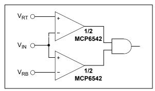
FIGURE 4-10: Windowed Comparator.
