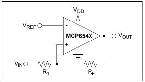
**FIGURE 4-3:** Non-inverting circuit with hysteresis for single-supply.
