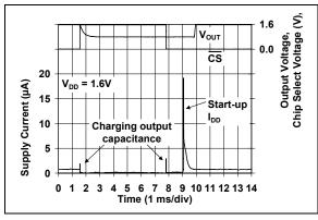
**FIGURE 2-33:** Supply Current (charging current) vs. Chip Select (CS) pulse at  $V_{DD} = 1.6V$  (MCP6543 only).
