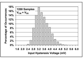
**FIGURE 2-4:** Input Hysteresis Voltage at  $V_{CM} = V_{SS}$ .
