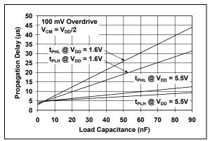
**FIGURE 2-31:** Propagation Delay vs. Load Capacitance.
