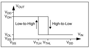
FIGURE 4-6: Hysteresis Diagram for the Inverting Circuit.
