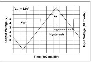
FIGURE 4-2: The MCP6541/2/3/4 comparators' internal hysteresis eliminates output chatter caused by input noise voltage.
