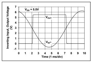
FIGURE 2-3: The MCP6541/2/3/4 comparators show no phase reversal.
