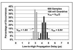
FIGURE 2-24: Low-to-High Propagation Delay.
