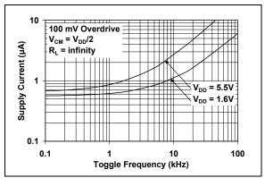
**FIGURE 2-19:** Supply Current vs. Toggle Frequency.
