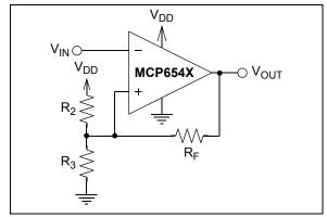
FIGURE 4-5: Inverting Circuit With Hysteresis.
