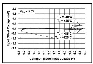
**FIGURE 2-9:** Input Offset Voltage vs. Common Mode Input Voltage at  $V_{DD} = 5.5V$ .
