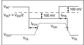
FIGURE 1-2: Propagation Delay Timing Diagram.
