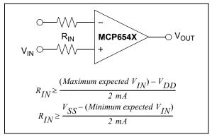
**FIGURE 4-1:** Input Current Limiting Resistor (R<sub>IN</sub>).
