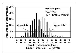
**FIGURE 2-5:** Input Hysteresis Voltage Linear Temp. Co.  $(TC_1)$  at  $V_{CM} = V_{SS}$ .
