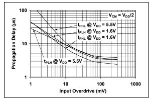
**FIGURE 2-29:** Propagation Delay vs. Input Overdrive.
