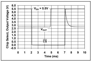
**FIGURE 2-34:** Chip Select ( $\overline{\text{CS}}$ ) Step Response (MCP6543 only).
