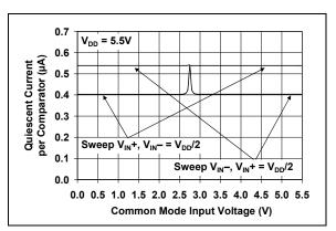
**FIGURE 2-18:** Quiescent Current vs. Common Mode Input Voltage at  $V_{DD} = 5.5V$ .
