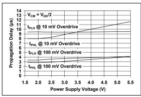
**FIGURE 2-26:** Propagation Delay vs. Power Supply Voltage.
