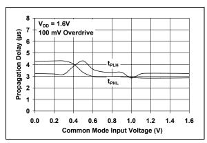
**FIGURE 2-27:** Propagation Delay vs. Common Mode Input Voltage at  $V_{DD} = 1.6V$ .
