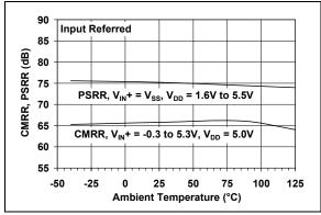
**FIGURE 2-13:** CMRR,PSRR vs. Ambient Temperature.
