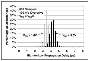
**FIGURE 2-21:** High-to-Low Propagation Delay.
