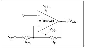
FIGURE 4-7: Thevenin Equivalent Circuit.
