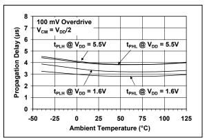
**FIGURE 2-28:** Propagation Delay vs. Ambient Temperature.
