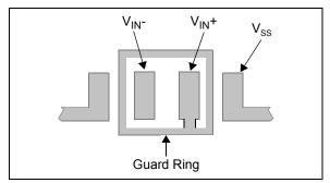
**FIGURE 4-8:** Example Guard Ring Layout for Inverting Circuit.
