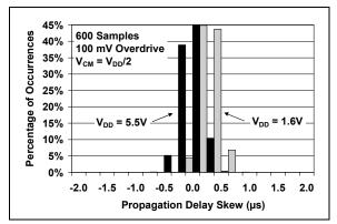
FIGURE 2-25: Propagation Delay Skew.
