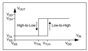
**FIGURE 4-4:** Hysteresis Diagram for the Non-Inverting Circuit.
