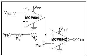
FIGURE 4-9: Precise Inverting Comparator.
