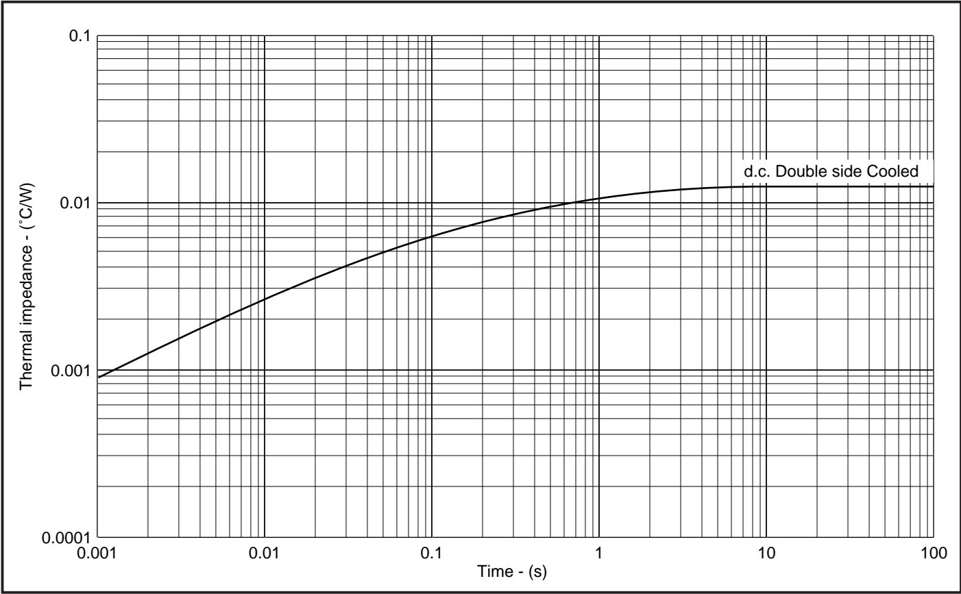
Fig.5 Maximum (limit) transient thermal impedance - junction to case - ( ^{\circ}\text{C/W} )
