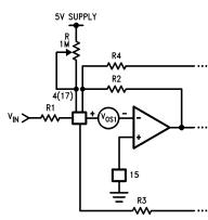
FIGURE 20. Method for Trimming  $V_{OS}$
