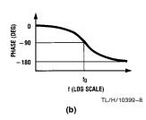
$$\begin{split} & H_{LP}(s) = \frac{H_{OLP}\omega_{O}^{2}}{s^{2} + \frac{s\omega_{O}}{Q} + \omega_{O}^{2}} \\ & f_{C} = f_{O} \times \sqrt{\left(1 - \frac{1}{2Q^{2}}\right) + \sqrt{\left(1 - \frac{1}{2Q^{2}}\right)^{2} + 1}} \\ & f_{p} = f_{O} \sqrt{1 - \frac{1}{2Q^{2}}} \\ & H_{OP} = H_{OLP} \times \frac{1}{\frac{1}{Q}\sqrt{1 - \frac{1}{4Q^{2}}}} \end{split}$$
