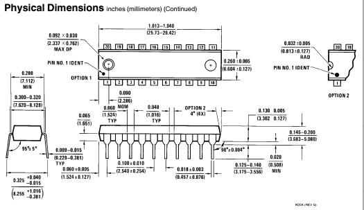
20-Lead Molded Dual-In-Line Package (N) Order Number MF10ACN or MF10CCN NS Package Number N20A
