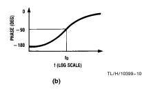
$$\begin{split} & H_{HP}(s) = \frac{H_{OHP} s^2}{s^2 + \frac{s\omega_O}{Q} + \omega_O ^2} \\ & f_C = f_O \times \bigg[ \sqrt{\bigg( 1 - \frac{1}{2Q^2} \bigg) + \sqrt{\bigg( 1 - \frac{1}{2Q^2} \bigg)^2 + 1}} \, \bigg]^{-1} \\ & f_p = f_O \times \bigg[ \sqrt{1 - \frac{1}{2Q^2}} \bigg]^{-1} \\ & H_{OP} = H_{OHP} \times \frac{1}{\frac{1}{Q} \sqrt{1 - \frac{1}{4Q^2}}} \end{split}$$
