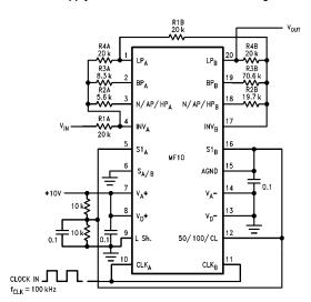
FIGURE 17. Fourth-Order Chebyshev Low-Pass Filter from Example in 3.1. Single  $\pm$  10V Power Supply. 0V–5V TTL Logic Levels. Input Signals Should be Referred to Half-Supply or Applied through a Coupling Capacitor.
