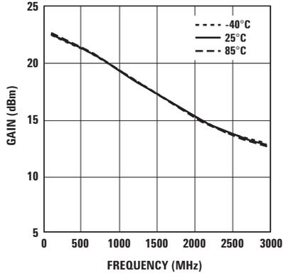
Figure 20. Gain vs. Frequency (5V 30 mA).
