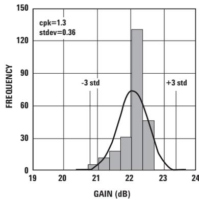
Figure 3. Gain @ 0.5 GHz 3V 60 mA. USL=23.4, Nominal=20.4, LSL=22.0.
