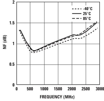
Figure 21. NF vs. Frequency (5V 30 mA).
