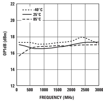
Figure 15. OP1dB vs. Frequency (3V 30 mA).
