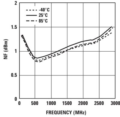
Figure 13. NF vs. Frequency (3V 30 mA).
