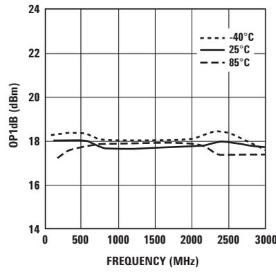
Figure 11. OP1dB vs. Frequency (3V 60 mA).
