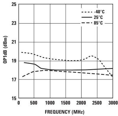
Figure 19. OP1dB vs. Frequency (5V 60 mA).
