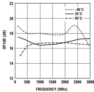
Figure 23. OP1dB vs. Frequency (5V 30 mA).
