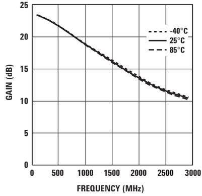
Figure 8. Gain vs. Frequency (3V 60 mA).
